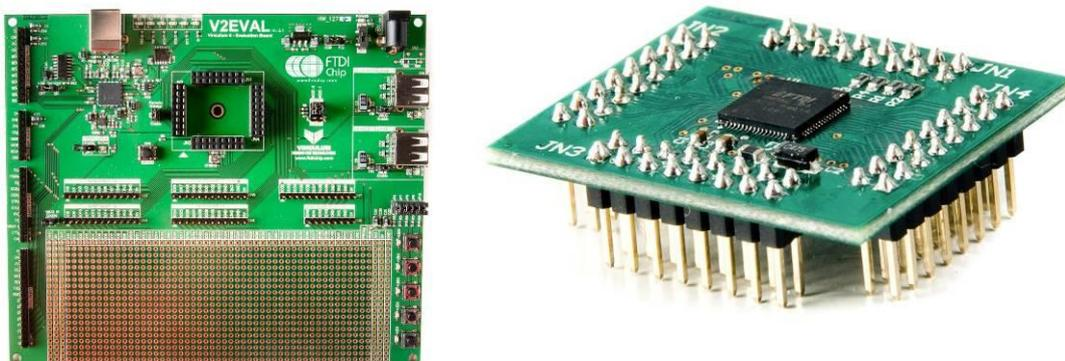
Figure 1.1 : V2-EVAL Motherboard(left) with Daughterboard Module(right)
