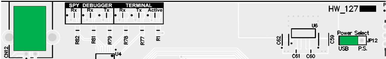
Figure 5.1 : Power Select Jumper Configuration for USB Power
