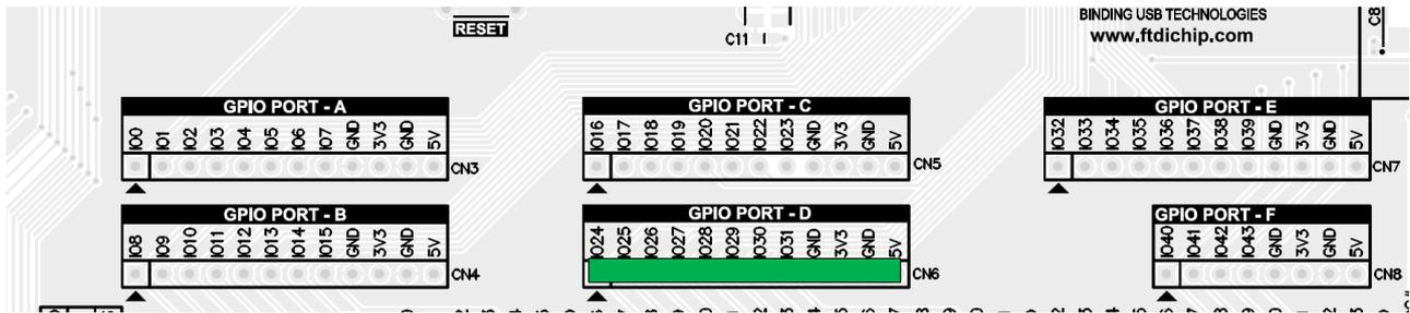
Figure 5.5 : GPIO[24:31] Connector CN6
