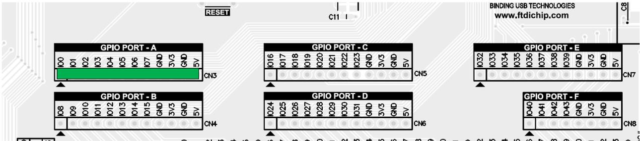
Figure 5.2 : GPIO[0:7] Connector CN3
