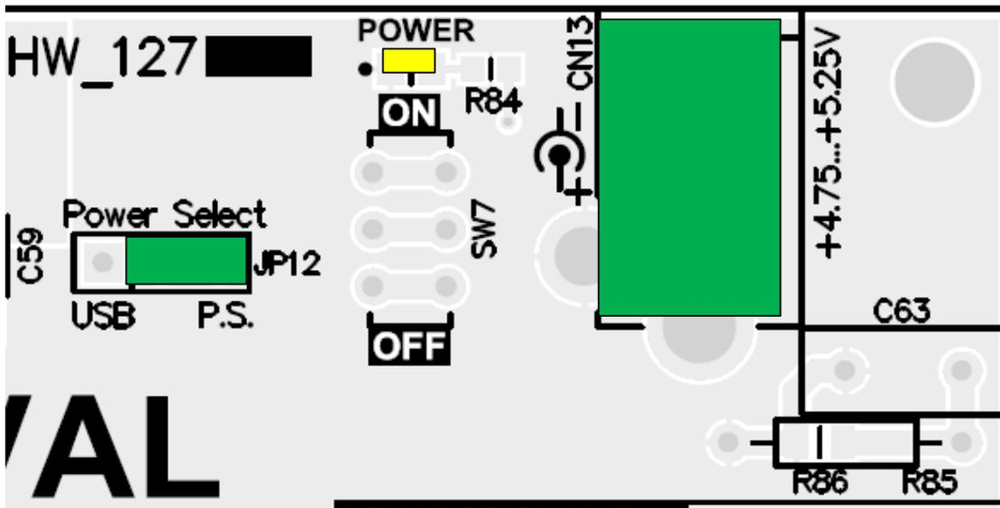
Figure 4.2 : Power connector with Jumper JP2
