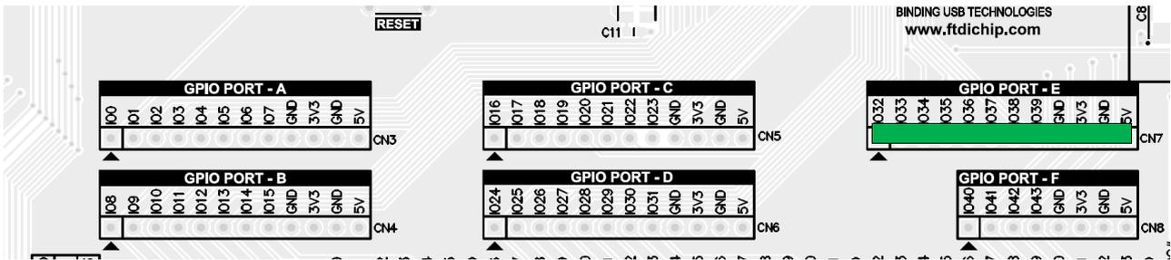
Figure 5.6 : GPIO[32:39] Connector CN7
