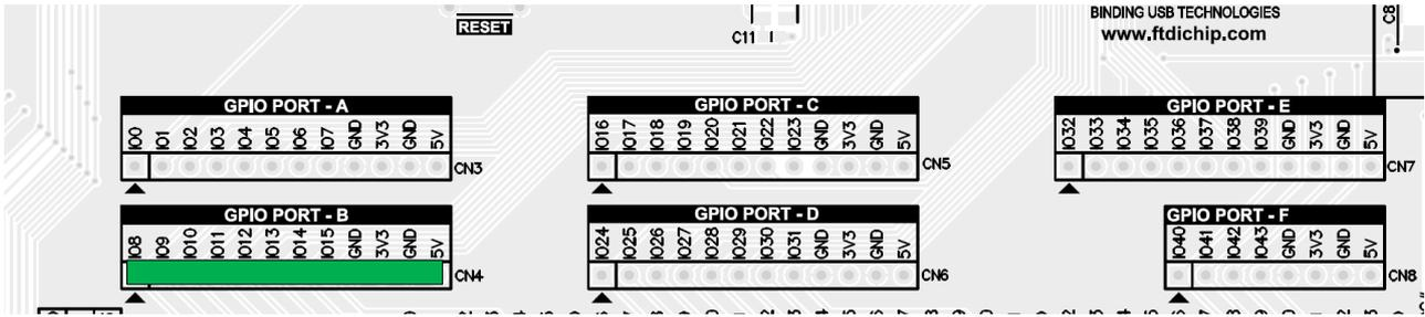
Figure 5.3 : GPIO[8:15] Connector CN4
