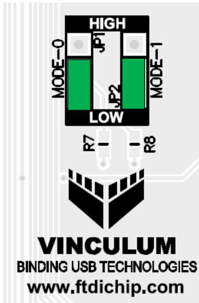
Figure 5.14 : GPIO Jumper pins, JP1, JP2
