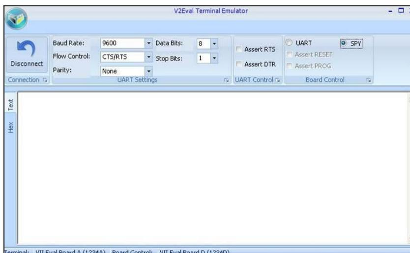
**Figure 8.4 : V2-EVAL Terminal connection with 'Spy' connection enabled**
