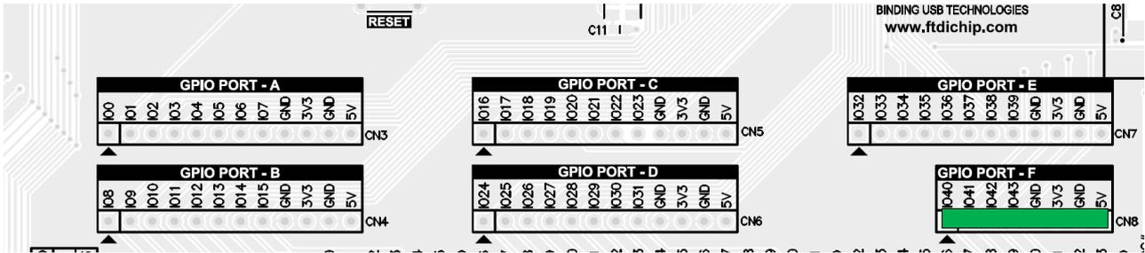
Figure 5.7 : GPIO[32:39] Connector CN8
