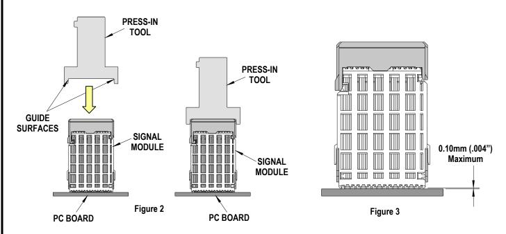
3. Using the application tool and an appropriate press, seat the vertical signal module until there is less than 0.10mm (.004 in) clearance between the bottom of the plastic housing and the surface of the PCB. See Figure 3.
