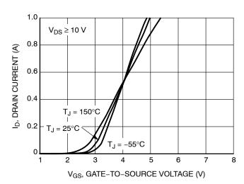
Figure 4. Transfer Characteristics
