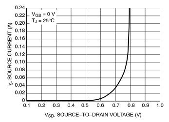
Figure 7. Diode Forward Voltage vs. Current
