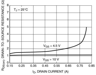
Figure 5. On-Resistance vs. Drain Current and Gate Voltage
