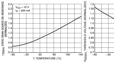
Figure 8. Temperature versus Static Drain-Source On-Resistance
