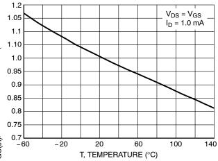
Figure 9. Temperature versus Gate Threshold Voltage
