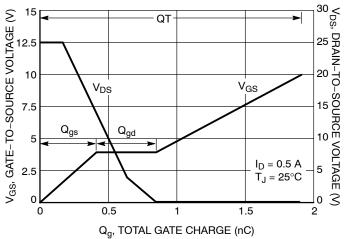
Figure 6. Gate-to-Source and Drain-to-Source Voltage vs. Total Charge
