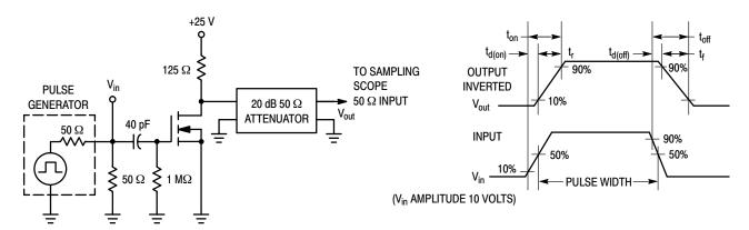
Figure 1. Switching Test Circuit
