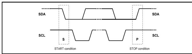
Both SDA data and SCL clock lines remain HIGH when the bus is not busy.
