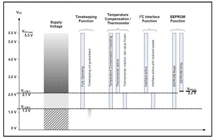
At first power-up, the supply voltage has to exceed V<sub>LOW1</sub> threshold to enable and correctly setup all function of the device.
