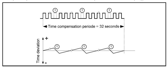
① **Time compensation cycle 32 seconds**: within a time compensation cycle of 32 seconds, the required numbers of 32.768kHz clocks are periodically suppressed (or added) to compensate the anticipated deviation of 32.768kHz reference clock.
