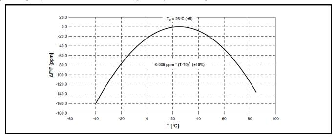
Above graph shows the typical frequency-deviation of a 32.768kHz "Tuning-Fork" Crystal over temperature. The parabolic curve is specified in terms of turnover temperature " $T_0$ " and the quadratic thermal coefficient " $\beta$ ".
