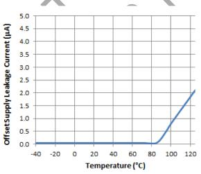
Figure 26. Offset Supply Leakage Current vs. Temperature
