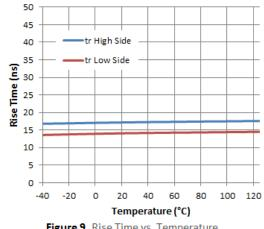
Figure 9. Rise Time vs. Temperature
