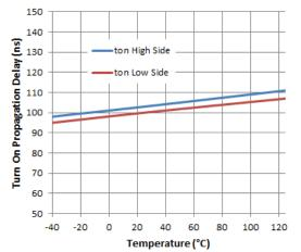
Figure 5. Turn-on Propagation Delay vs. Temperature
