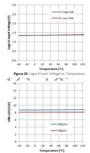
Figure 25. VBS UVLO vs. Temperature
