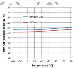
Figure 7. Turn-off Propagation Delay vs. Temperature
