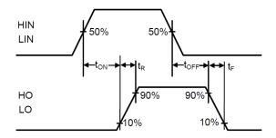
Figure 2. Switching Time Waveform Definitions
