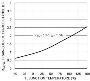
Figure 7. On-Resistance Variation with Temperature
