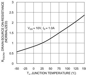
Figure 6. On-Resistance Variation with Temperature
