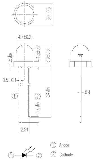
Note: Tolerances unless dimensions ±0.25mm
