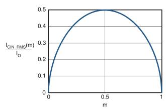
Figure 2. I<sub>CIN</sub> vs. Voltage Conversion Ratio
