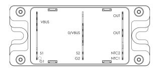
$V_{DSS} = 900V$   $R_{DSon} = 60m\Omega \text{ max } @ \text{Tj} = 25^{\circ}\text{C}$  $I_D = 59\text{A} @ \text{Tc} = 25^{\circ}\text{C}$
