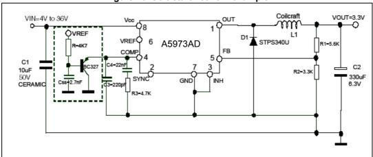
Figure 26. Soft-start network example
