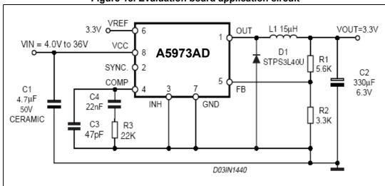
Figure 18. Evaluation board application circuit
