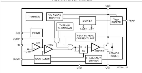
Figure 3. Block diagram
