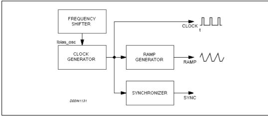
Figure 5. Oscillator circuit block diagram
