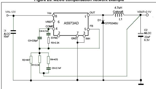
Figure 25. MLCC compensation network example
