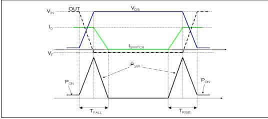
Figure 14. Switching losses
