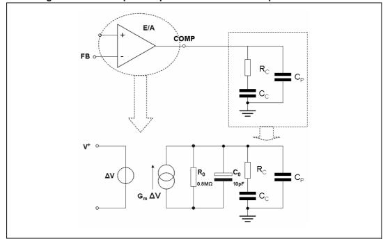
Figure 10. Error amplifier equivalent circuit and compensation network
