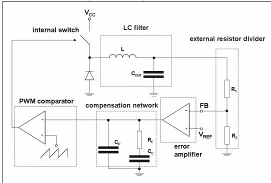
Figure 9. Block diagram of the loop
