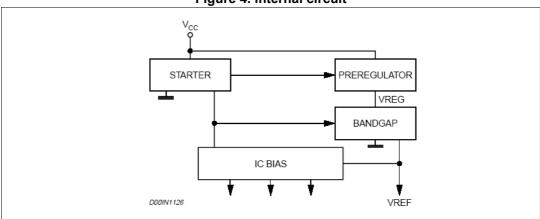
Figure 4. Internal circuit
