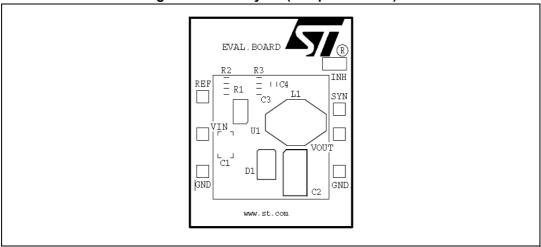
Figure 20. PCB layout (bottom side)
